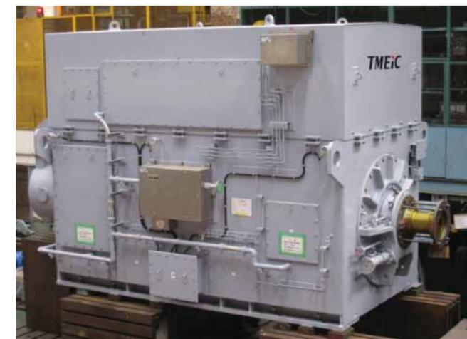
High Speed 25 MW 3,780 rpm Synchronous Motor
