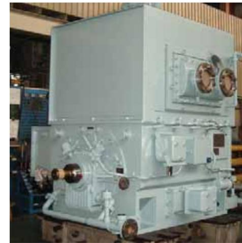
11,900 rpm, 1.8 MW, Induction Motor
