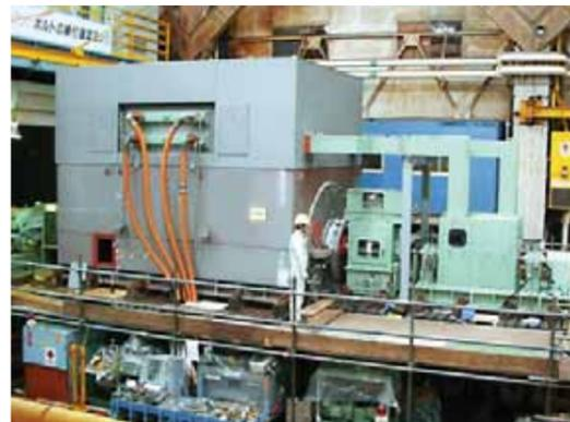
Up to 3,600 rpm, 53 MW, Synchronous Motor
