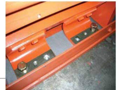
TMEIC unique spring-mounted stator design reduces vibration
