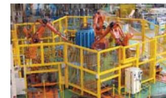
Robotic Stator Core Lamination Stacking
